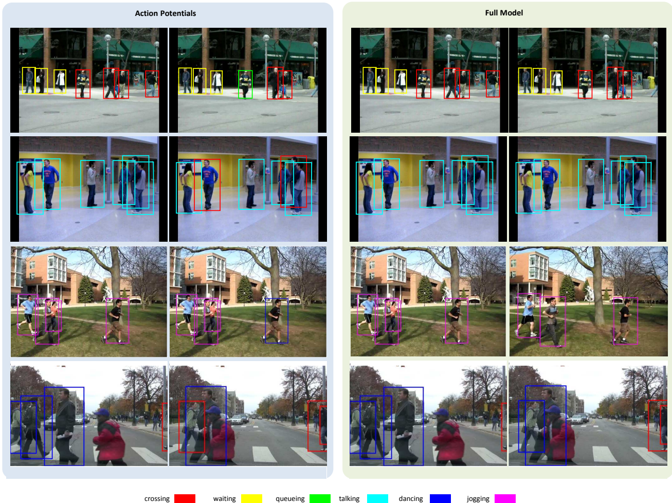
Figure 5. Qualitative results with and without our full model. The first two columns are the results of two consecutive frames from the same video sequence using only the action potentials, and the next two columns are the results of the same two frames, but using our full model. Each row represents a different video sequence. The first row shows a video sequence where the misclassification of crossing as queueing is fixed with correct tracking. The second shows the same case for talking being misclassified as crossing , and the third for jogging being misclassified as dancing . The fourth row is a case where the full model actually decreases the classification accuracy due to the high confidence of the action classifier in the wrong label.
