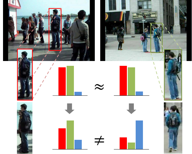
Figure 1. How tracking can improve action recognition. While the person outlined on the left is queueing and the person outlined on the right is waiting to cross, a classifier might initially return similar scores for both given the resemblance in their appearance and stance. However, the actions become more distinguishable after the person on the right is tracked to subsequent frames and is observed to be crossing. We present a framework to solve both problems jointly and efficiently.
