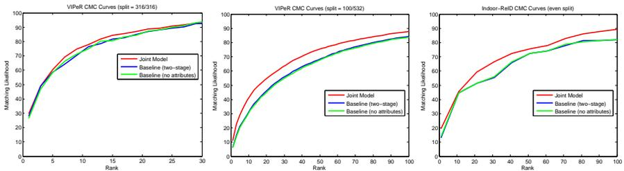
**Fig. 3.** CMC Curves for VIPeR and Indoor-ReID. The curve for the joint model using the coupled appearance-attribute space dominates the two baseline curves in all graphs. The first graph for VIPeR was created with an even training/test split (316/316), while the second graph figure was created with a split of 100 training subjects and 532 test subjects. For Indoor-ReID the dataset was split evenly.
